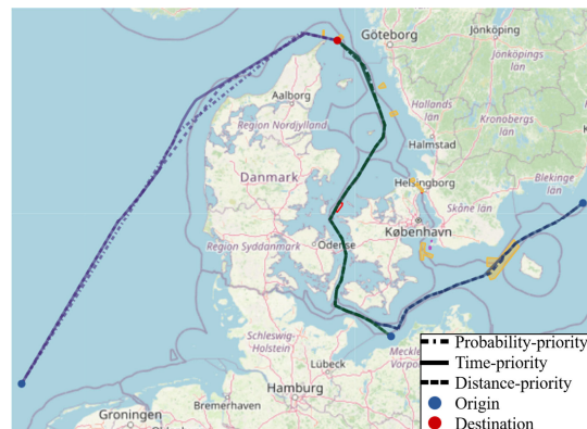
Fig. 11. Pathfinding results without local refinement for the tanker and Draft = 12 m (OD1: blue; OD2: purple; OD3: green).
