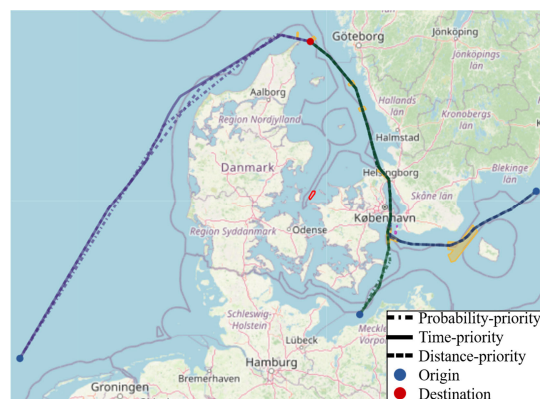
Fig. 10. Pathfinding results without local refinement for the tanker and Draft = 6 m (OD1: blue; OD2: purple; OD3: green).
