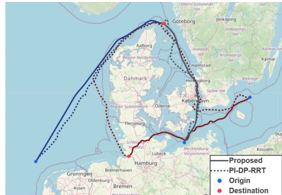
Fig. 12. Representative routes produced by the proposed framework (with local refinement) and PI-DP-RRT for OD2 (blue), OD4 (red), and OD5 (grey).
