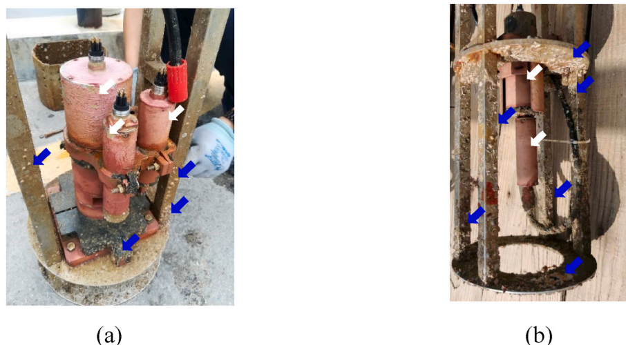
Fig. 5. Application of the CPT-based paint on housings of the COD sensor, the Chl a sensor and their wiper for 4 months (a) and on the housing of the BOD sensor for 6 months (b). White arrows indicate the instrument housings painted with CPT-based paint, and blue arrows indicate unpainted frames with fouling organisms settled on their surfaces. (For interpretation of the references to colour in this figure legend, the reader is referred to the Web version of this article.)
