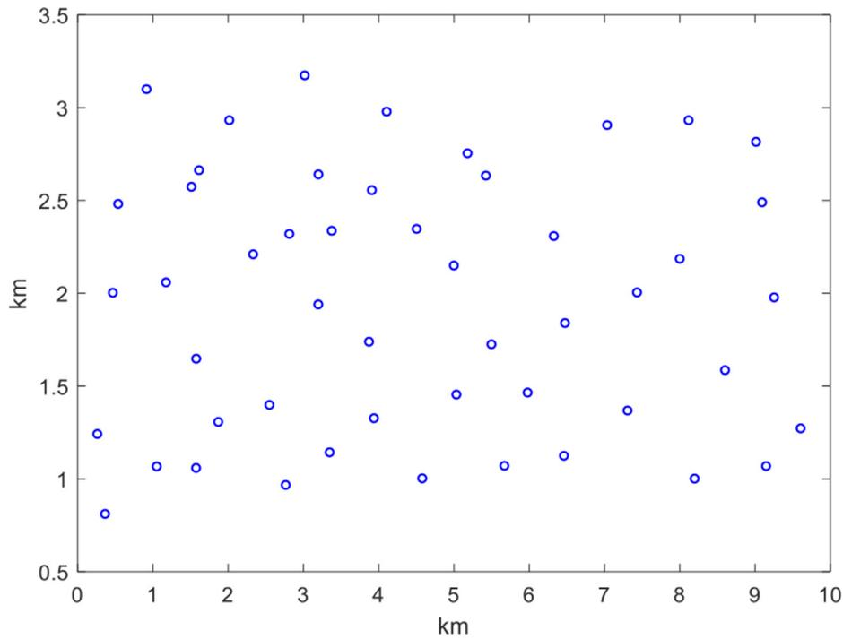
Fig. 6. Network topology of an UASN with 50-node.
