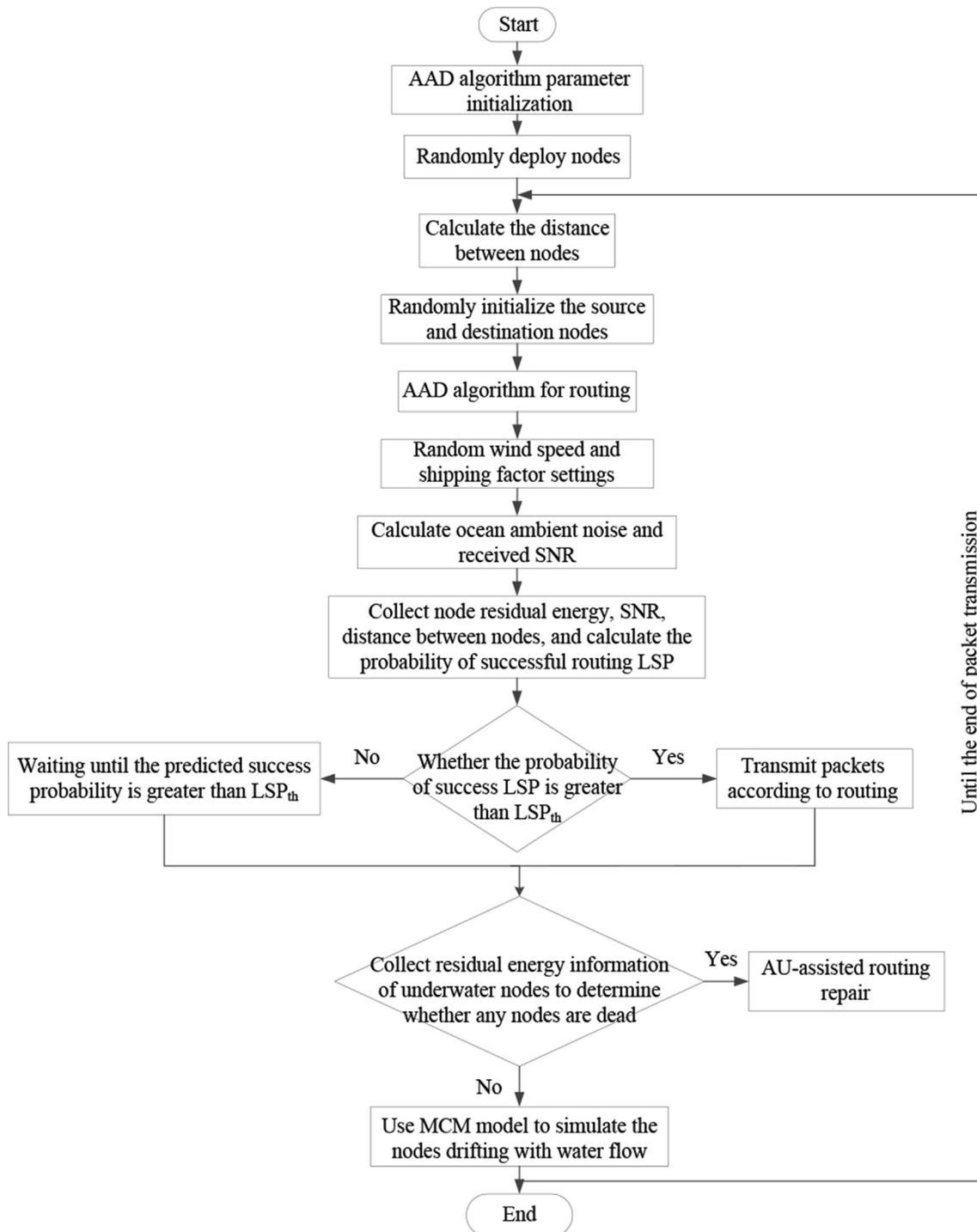
Fig. 3. AAD-FPVR algorithm flow diagram.
