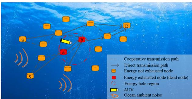
Fig. 1. Application scenario of an AUV-assisted UASN.
