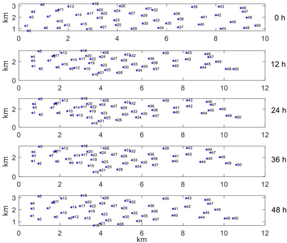
Fig. 7. The change process of the position of the underwater sensor node over time.
