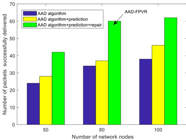
Fig. 12. Comparison of the number of packets successfully delivered between the algorithm with the repair mechanism and the original ADD algorithm.
