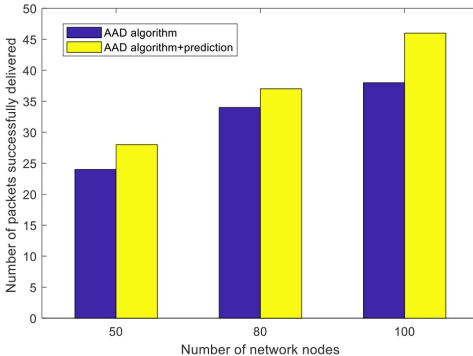
Fig. 11. Comparison of the number of packets successfully delivered by the original AAD algorithm and the AAD algorithm incorporating link failure prediction mechanism.
