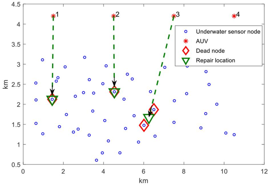
Fig. 8. Network topology after AUV-assisted repair.
