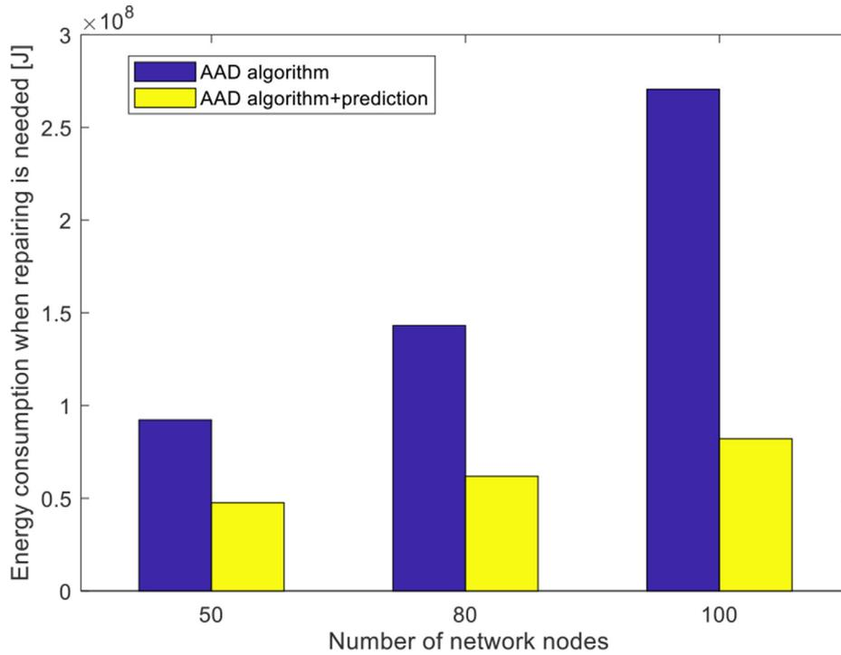
Fig. 10. Comparison of energy consumption between the original AAD algorithm and the AAD algorithm incorporating link failure prediction mechanism.
