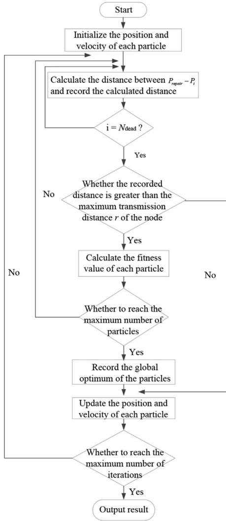
Fig. 5. Flow chart of PSO algorithm.
