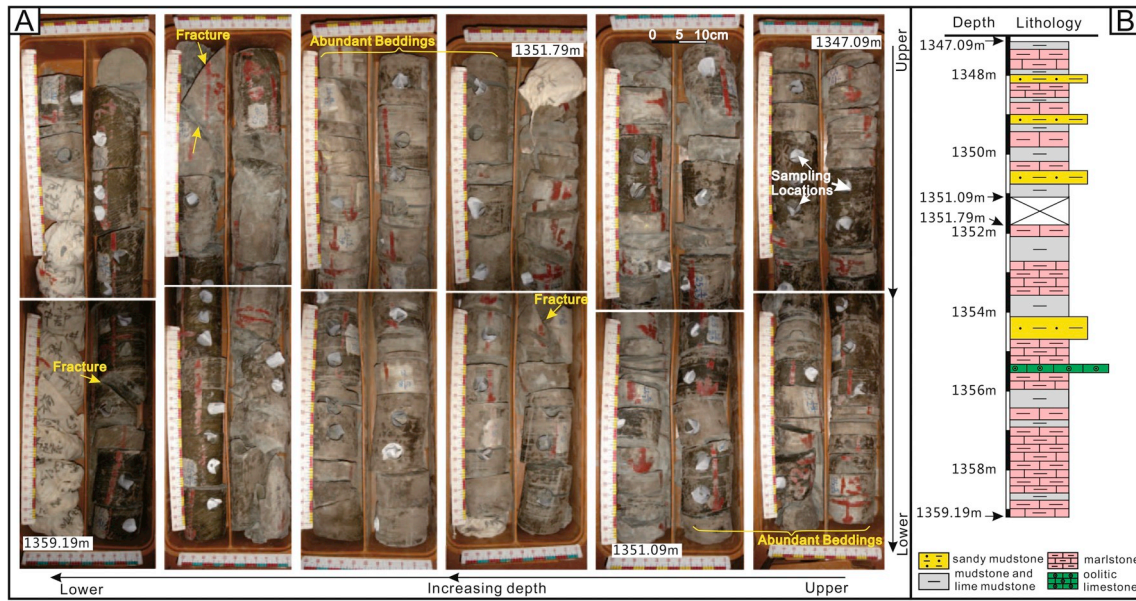
Fig. 2. Representative rock cores (A) and the corresponding lithology column (B) of Well L101 in the Xiaoliangshan area. The lithology column is based on on-site core description. The illustrated rock cores, which are mainly composed of marlstones and mudstones, were collected from 1347.09 m to 1359.19 m (N 2 2 ). The marlstones are characterized by macro-fractures (marked by yellow arrows) and show black and dark grey in colors, while the mudstones are characterized by abundant horizontal millimeter-scale laminations and show grey in colors. (For interpretation of the references to color in this figure legend, the reader is referred to the Web version of this article.)
