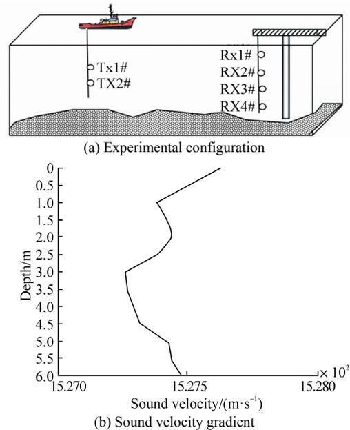
Fig. 2 Experimental configuration of MIMO acoustic communication system
