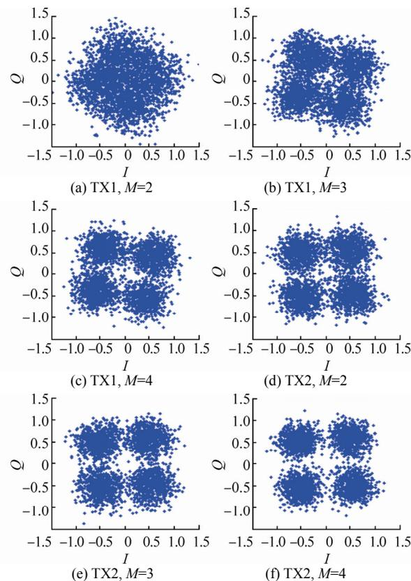
**Fig. 5 Scatter plots of MIMO multichannel TR receivers with different number of receiving elements**
