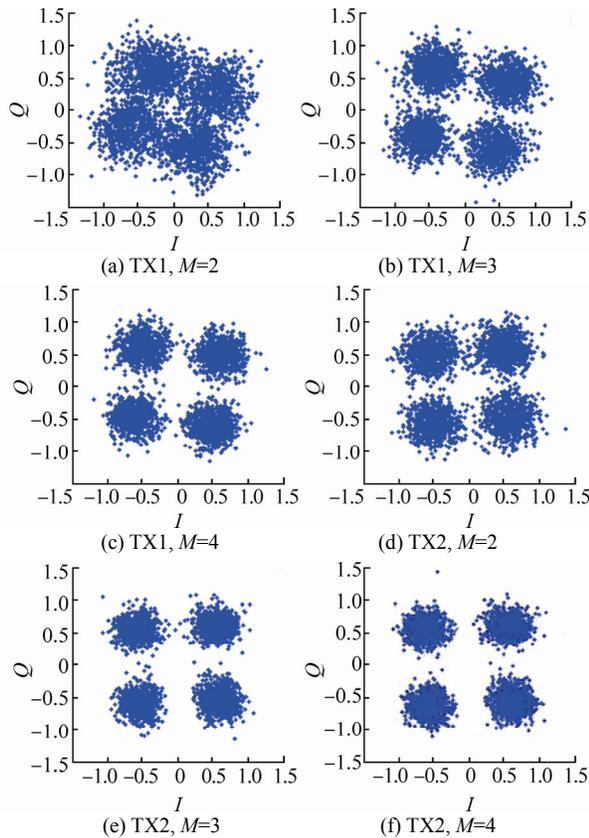
**Fig. 4 Scatter plots of MIMO multichannel DFE receivers with different number of receiving elements**
