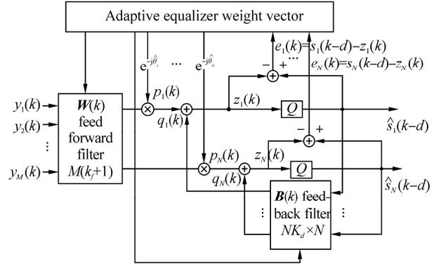
Fig. 1 Illustration of the multichannel DFE receiver
