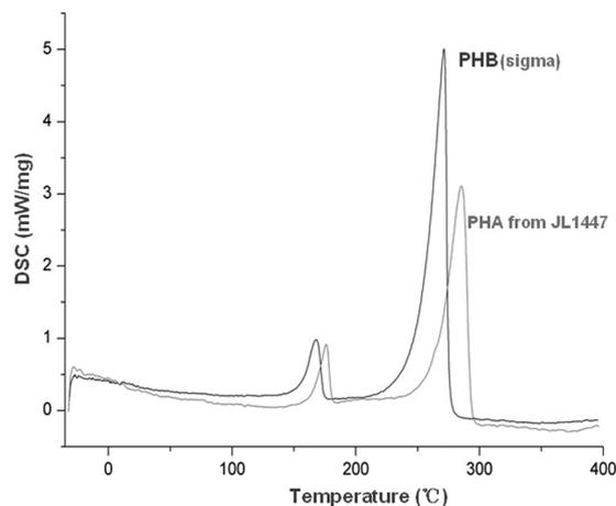
FIG. 3. DSC spectra of PHB standard and PHA produced by *Dinoroseobacter* sp. JL1447. The  $T_m$ ,  $\Delta H_m$ , and  $T_d$  values of the sample are 175.8°C, 51.87  $\text{J g}^{-1}$ , and 285°C, respectively, which are very close to those of the PHB standard (167.8°C, 58.3  $\text{J g}^{-1}$ , and 272°C).
