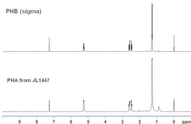
FIG. 2.  $^1\text{H}$  NMR spectra of PHB standard and PHA produced by *Dinoroseobacter* sp. JL1447. The spectra show peaks of  $\text{HC}=\text{CH}$  bonds at 5.30 ppm,  $\text{CH}_2\text{—COOH}$  bonds at 2.50 ppm, a  $-\text{CH}_2$  group in the saturated lateral chain at 1.28 ppm, and a terminal  $-\text{CH}_3$  group at 0.9 ppm.
