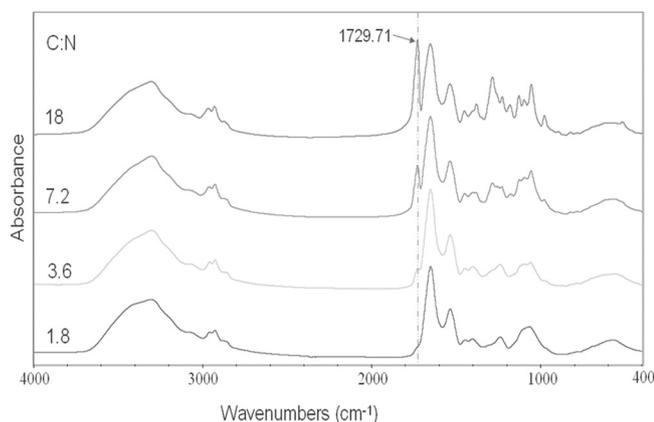
FIG. 5. FTIR spectra of *R. denitrificans* OCh 114 cultured in media with different C/N ratios. The medium was adjusted with glucose at different concentrations, with NH<sub>4</sub>Cl at a fixed concentration of 0.25 g liter<sup>-1</sup>, and the spectra indicate the increase of the PHA signal with increasing C/N ratios.
