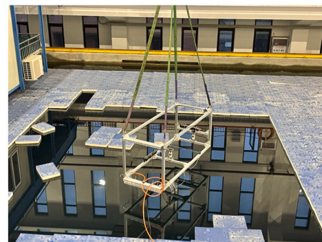
Fig. 3. Experimental scenario. The aluminum alloy frame carrying acoustic devices and air stones was suspended by a crane.
