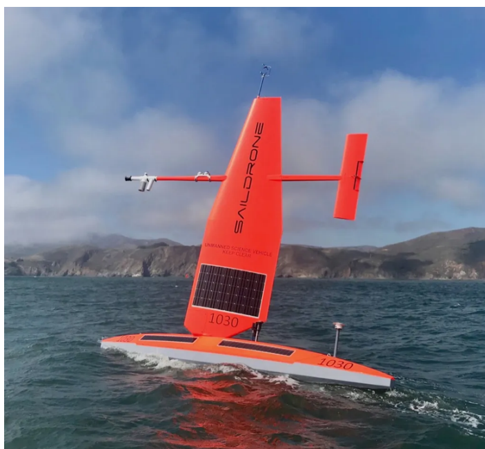
Photo of a saildrone, an autonomous sailing drone used to collect high quality oceanic and atmospheric observations. Credit: NOAA
