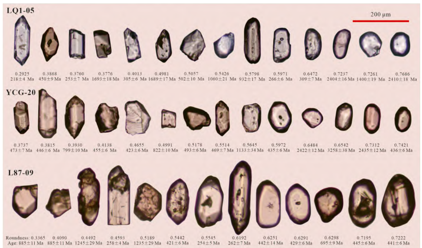
Fig. 25. Textural features (under plane-polarized light) of representative dated detrital zircon grains of three Cenozoic sandstone samples from the northern Qaidam basin. The zircon roundness was quantified through a mathematical method proposed by Resentini et al. (2018) based on image analysis, following the procedures given by Shen et al. (2021). Note that the roundness values of most analyzed zircon grains range from 0.2 to 0.8, revealing that the zircon grains in the Cenozoic northern Qaidam basin are subangular to well-rounded in shape (Shen et al., 2021).
