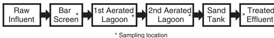
Fig. 1. Schematic diagram of the rural wastewater treatment facility.
