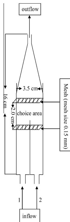
**Fig. 1.** The draft of two channel flume (length 16 cm, width 3.5 cm) used in pH sensitivity test. The numbers “1” and “2” are two inlets that were separately connected to the transfusion bags which store the seawater. Two meshes were put in the channel to form a choice area (3.5 cm  $\times$  2 cm) in which the high- and low- $\text{CO}_2$  water can be distinguished based on the dye test. Not drawn to scale.
